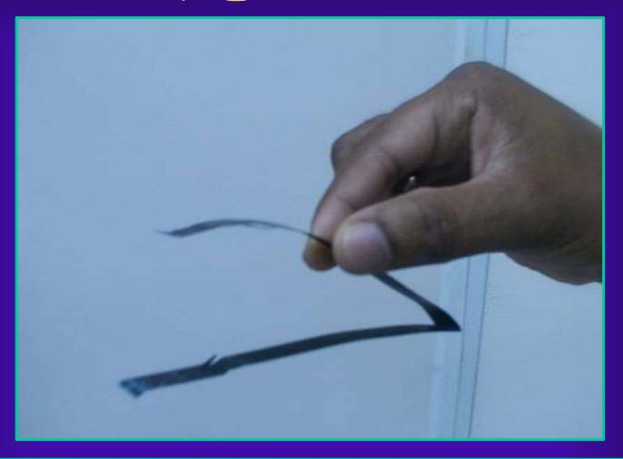
• The trap is made up of XRAY film, which is the preferred material by thieves; Simply because of the black color which is similar in appearance to the slot on the card reader.
