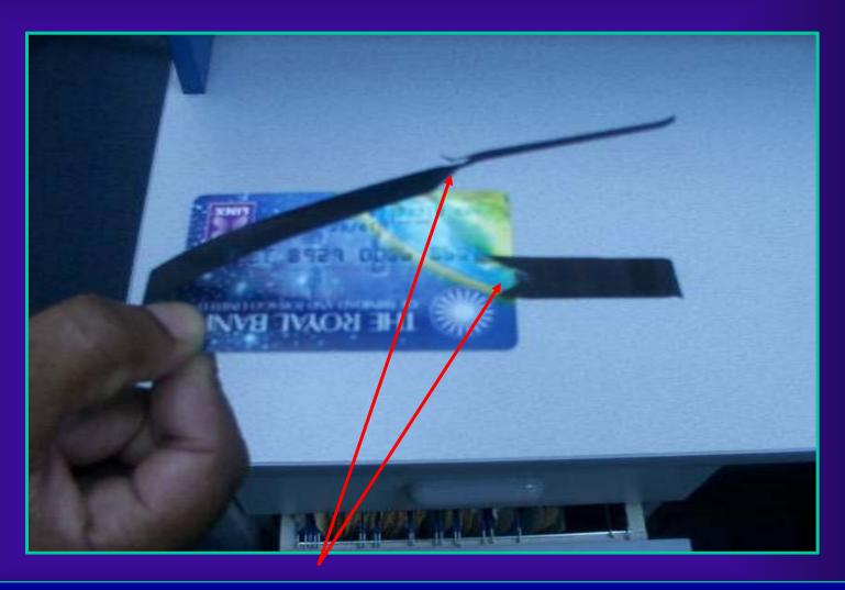
Slits are cut into both sides of the trap, This prevents your card being returned prior to completing your transaction.
