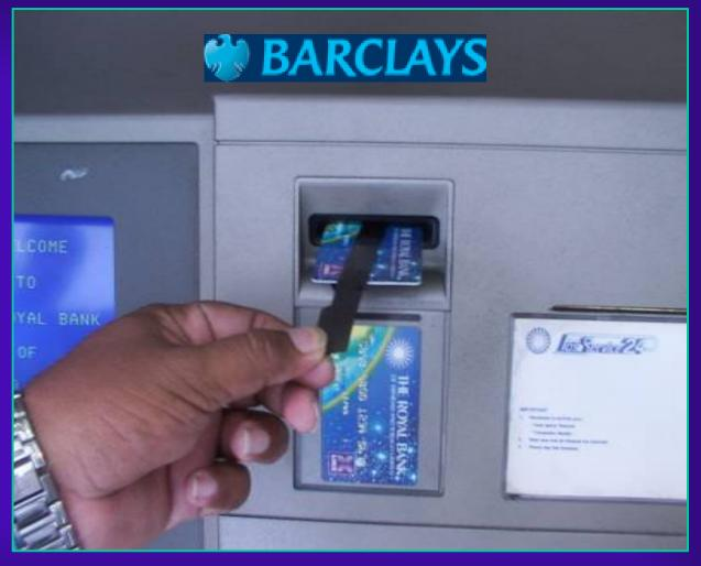
• As soon as the "Customer" has gone, and they have your PIN, The thief can remove the glued trap, by grasping the folded tips, he simply pulls the trap out that has retained your card..
